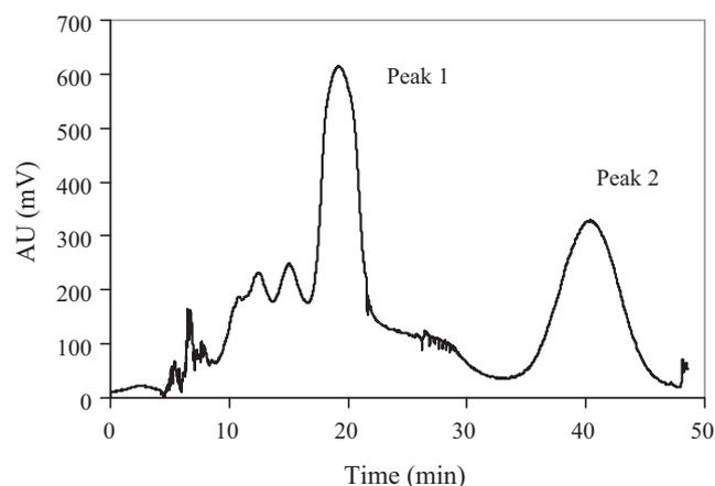
**Fig. 2.** First separation stage of cryptotanshinone and tanshinone IIA on Mini HPCCC using hexane–dichloromethane–methanol–water (4:0.75:4:1) solvent system; loading 20 mg in 0.8 mL upper phase; flow rate 1.0 mL/min; rotation speed 2100 rpm (Peak 1, Cryptotanshinone with contaminant; Peak 2, Tanshinone IIA).  $S_f = 68.6\%$ .
