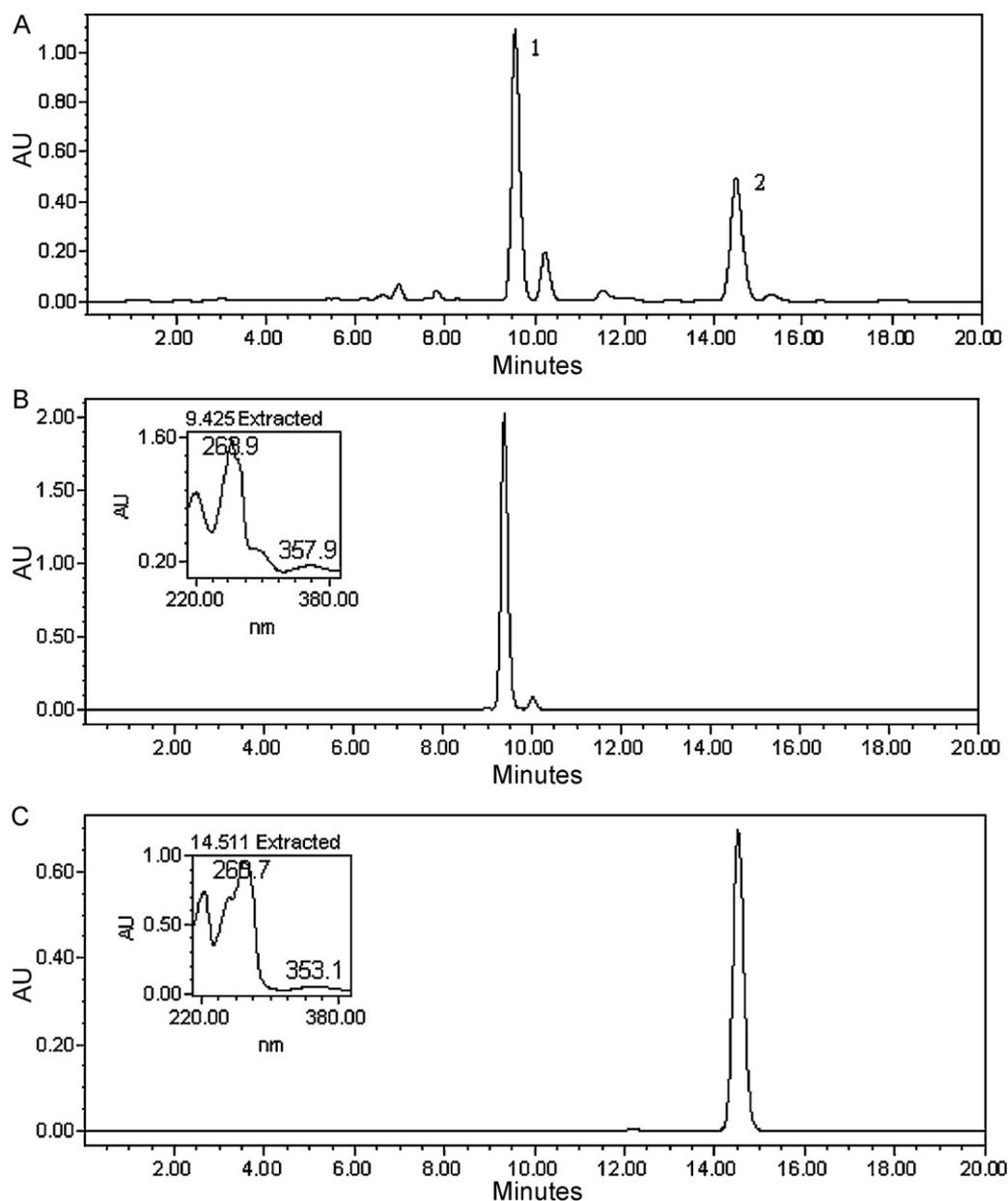
**Fig. 6.** HPLC chromatogram of crude A (A), purified peak 1 (B), purified peak 2 (C). Alltima C18 column (250 mm × 4.6 mm i.d., 5 μm); column temperature 27 °C. solvent A, 0.05% aqueous trifluoroacetic acid and solvent B, acetonitrile; flow rate: 1.0 mL/min; isocratic elution 0–20 min, 75% B. wavelength 280 nm. (Peak 1, Cryptotanshinone; Peak 2, Tanshinone IIA).
