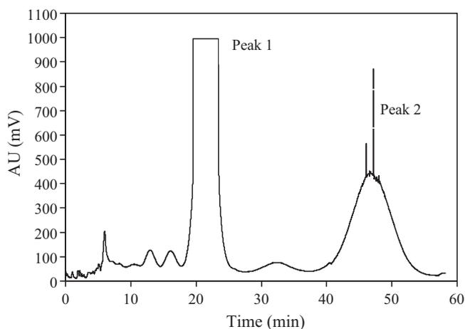
**Fig. 4.** First stage separation of cryptotanshinone and tanshinone IIA by Midi HPLCC using hexane–dichloromethane–methanol–water (4:0.75:4:1) solvent system; loading 700 mg in 50 mL upper phase; flow rate 45 mL/min; rotation speed 1250 rpm (Peak 1, cryptotanshinone with contaminant; Peak 2, tanshinone IIA).
