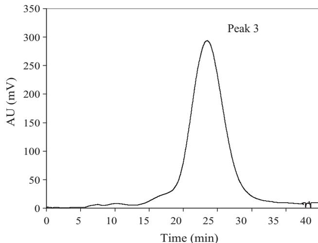
**Fig. 3.** Second purification stage of cryptotanshinone by Mini HPCCC using hexane–ethanol–water (4:2:2) solvent system, flow rate 0.5 mL/min; rotation speed 2100 rpm (Peak 3, cryptotanshinone).  $S_f = 79.1\%$ .
