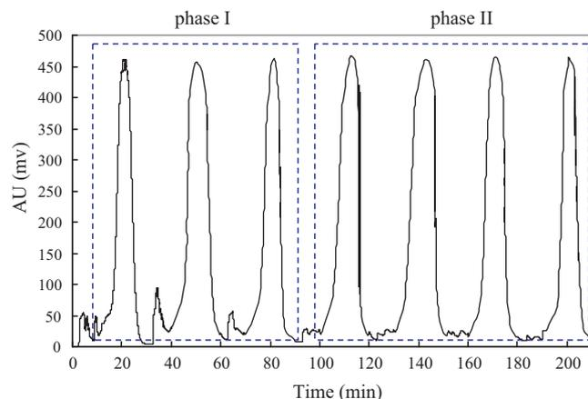
**Fig. 5.** Second purification stage of cryptotanshinone on Midi HPLCC by multi-injection using hexane–ethanol–water (4:2:2) solvent system, flow rate 25 mL/min; rotation speed 1250 rpm. *Sf* = 90.1%.
